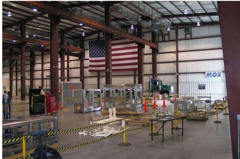
First Process Gloveboxes Being Assembled
